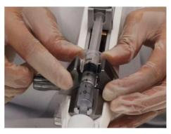
Tighten the hold down screw on the syringe holder until the syringe is snug against syringe holder.
