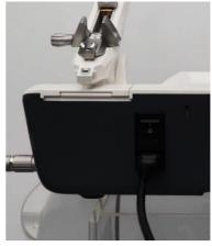
Open prepared filter. Install the filter into the filter groove on the right side of the injector.
