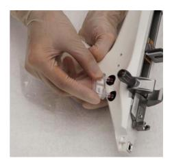
Prepare the disposable multi needle Align the injector vacuum hole with the multi needle vacuum hole then press down from top to bottom until it clicks.
