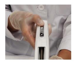
Position the syringe at the injector and push the end of the plunger downwards into the position holder.
