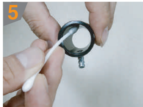
5 Clean interior of Ending Tip using soft cloth or Q-tip. Reassemble Hand Piece after cleaning.
