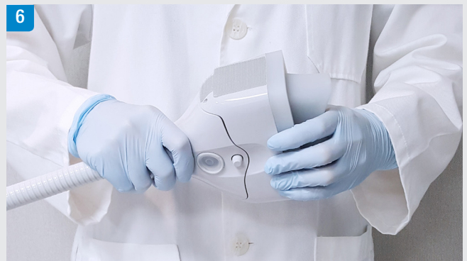
6 Connect the selected cooling cup to the handpiece. (Press down firmly until a clicking sound occurs.)
