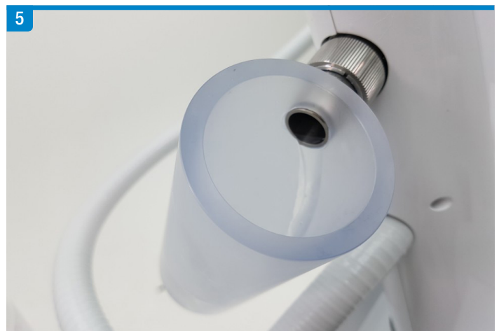
5 Check that the oil is draining properly through the input of the Oil Receiver. Keep the Oil Receiver connected until oil is completely drained from the System. After a successful drainage, remove the Oil Receiver from the Arm Stand in reverse sequence.
