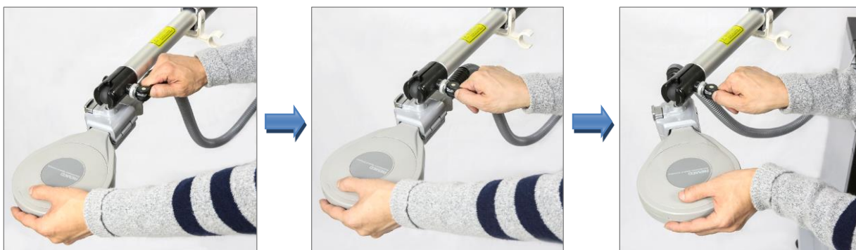
Figure 11. Changing the angle of the transducer
