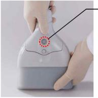
(1) Simultaneously press the two buttons on both sides of the Hand-piece for 2 seconds. LED signal displays a yellow light.
