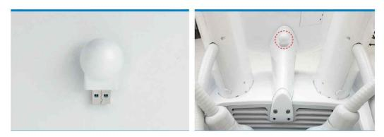
Figure 4.6 SAT Card connects into the USB port
