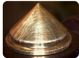
360° gold mirror with excessive scratches
