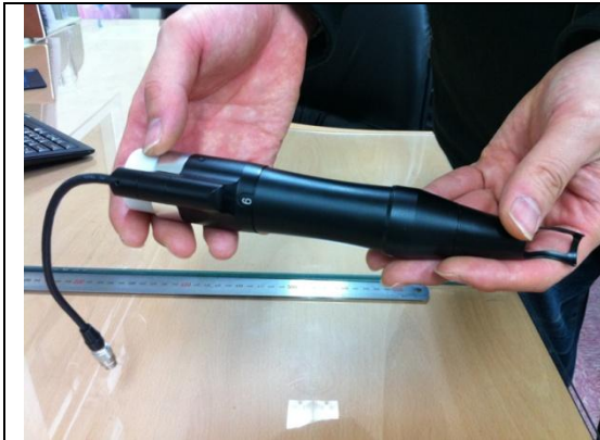
1) Twist out Handpiece from articulated arm
