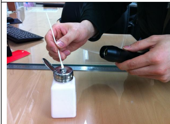
3) Preparing the cotton swab with alcohol
