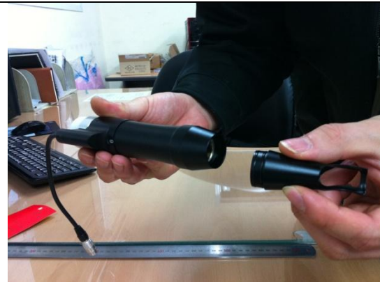
2) Pull out tip to detach it from Handpiece
