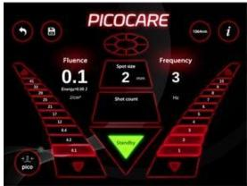
10) During radiation of treatment laser with aiming beam, if hazardous situations occurred, press the emergency switch to shut down the device. An alarm message appears on the screen. For returning in Standby mode, release the emergency switch.
