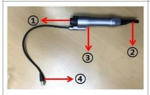
Picocare uses Zoom handpiece for operation at either 1064nm or 532nm. It provide a range of spot sizes by rotating the barrel of the handpiece and it overrides the spot size setting indicated on the screen.
