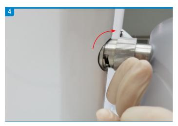
After the input of the Oil Receiver is inserted into the outlet, turn the input right to ensure a firm connection.
