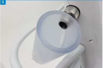
Check that the oil is draining properly through the input of the Oil Receiver.
