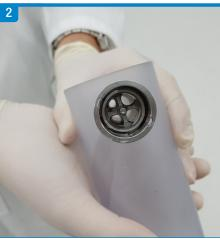
Prepare to connect the Oil Receiver to the outlet.
