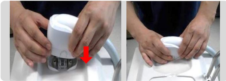
[Disconnection] Press the button in both sides of the handpiece and pull the connector upward.
