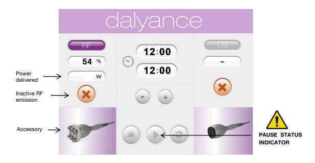
With the equipment in *Play Mode,* the radio frequency emission is activated by keeping one's foot *pressed on the pedal.*
