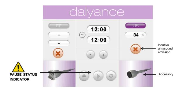
With the device in *play mode*, the ultrasound emission is activated by keeping one's foot *pressed on the pedal*.
