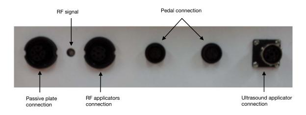
Use the connector for *ultrasound head connection* to connect the ultrasound accessory.
