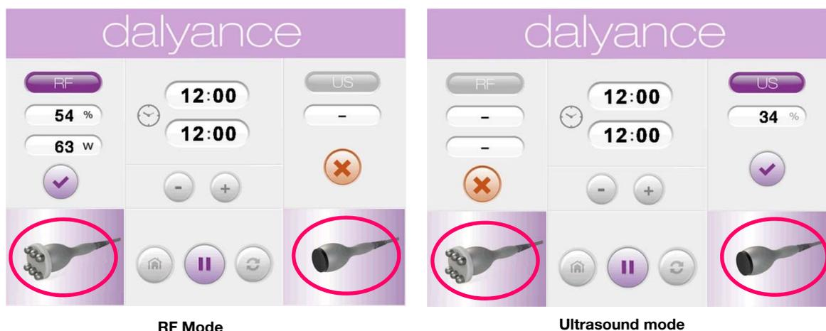
**The accessory detection** shows that both heads are connected and work settings can be selected for each work mode. To select and validate treatment settings, follow the detailed steps in sections **RF mode** and **ultrasound mode**.
