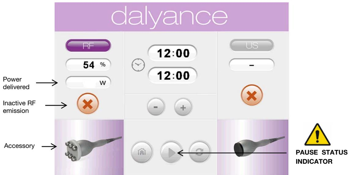
With the equipment in **Play Mode**, the radio frequency emission is activated by keeping one's foot **pressed on the pedal**.
