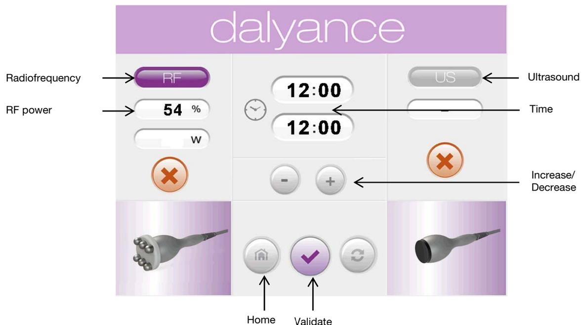
With **RF Mode** activated, the following is enabled:
